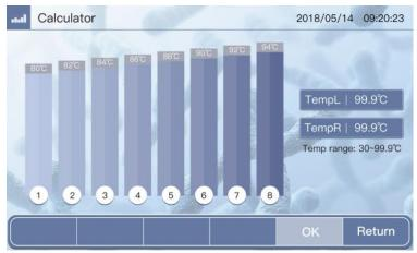
**b.** Press on the corresponding area and enter the module temperature and gradient range. After the input is complete, press "OK" to automatically calculate the temperature of each sample. Press "Return" to get to the main menu.
